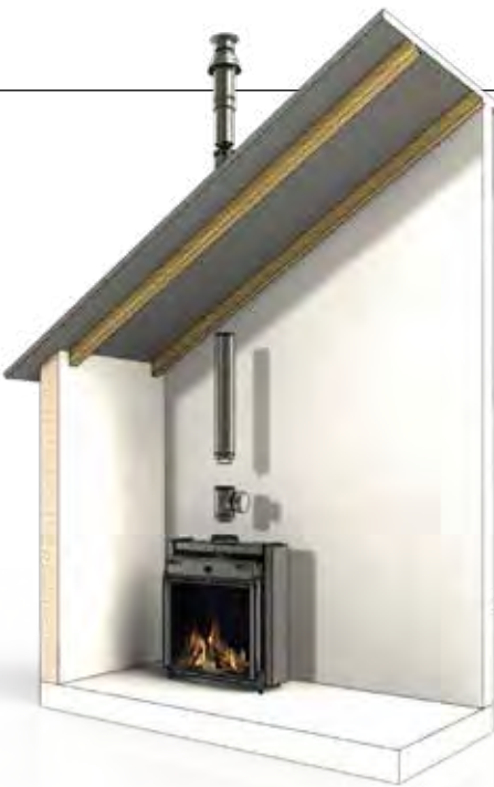
Via roof [pitched] • straight or with bends
